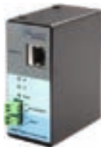
Modbus RTU, Modbus TCP, BACnet MSTP, BACnet IP, N2, SNMP, XML
